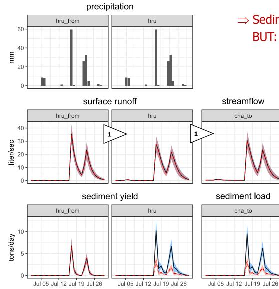
$\Rightarrow$  Sediment yield on grassed hru can be simulated (with usle\_p = 0.5) BUT: this is erosion, not sediment transport!
