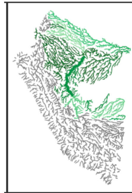
Ratio of floodplain width to bankfull width (FP_W_F = FP_W/W)
