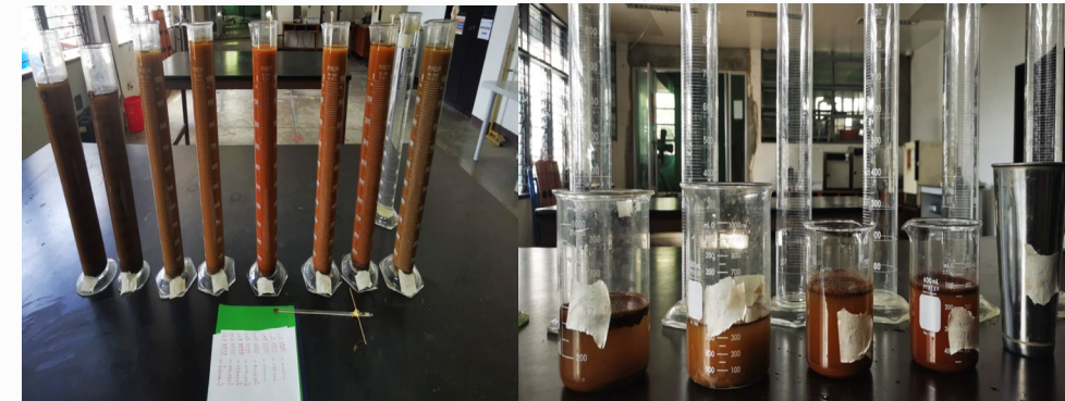
Figure: Soil Particle Size Analysis Using the Hydrometer Method
