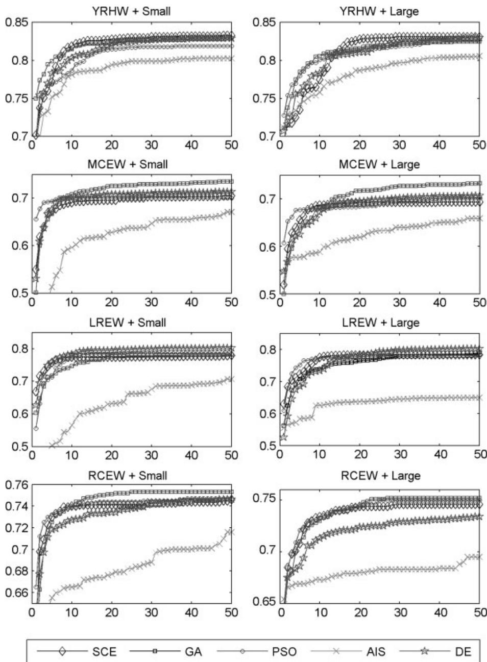
Figure 3. Performances of the different optimization algorithms versus number of evaluations in the four test watersheds (x axis represents the number of model evaluations  $\times$  200, y axis represents  $E_{ns}$  value)
