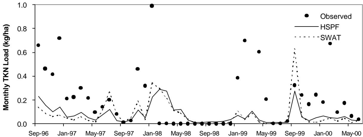
Figure 4. The observed and simulated monthly TKN loads at QPE during the calibration period
