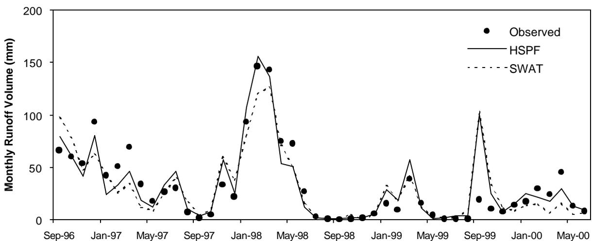
Figure 2. The observed and simulated monthly runoff volumes at QPE during the calibration period
