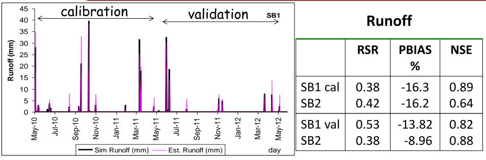
Comparisons between simulated and measured runoff during calibration and validation periods
