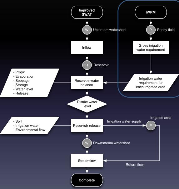
Watershed water balance using improved SWAT coupled with the IWRM models is performed by considering the relationship between upstream, downstream, and reservoir
