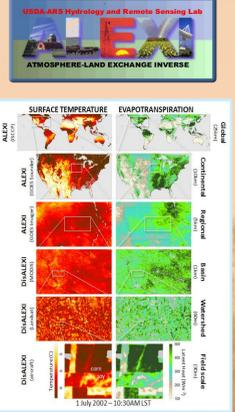
A two-source model (soil + vegetation) energy balance model is applied in a time differential mode, coupled with an atmospheric boundary layer (ABL) model to internally simulate land-atmosphere feedback on near-surface air temperature and surface fluxes. This reduces sensitivity to LST retrieval errors.
