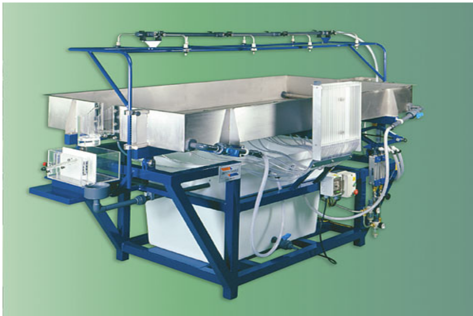
Fig.1 S-12 MKII-50 Advanced Hydrologic Systems (rainfall simulator).
