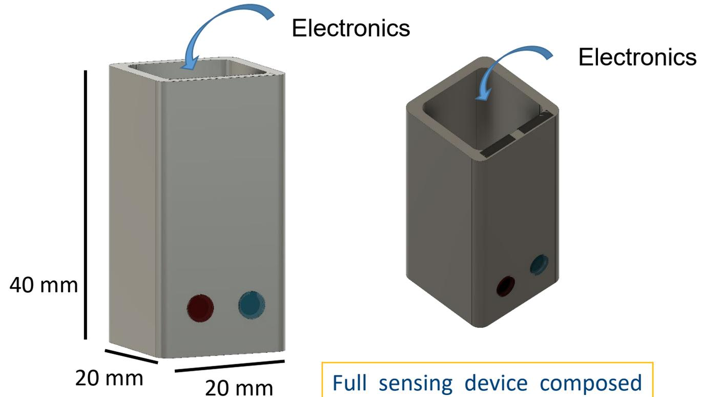
Full sensing device composed by nitrate-selective sensor, electronic board and communication system.
