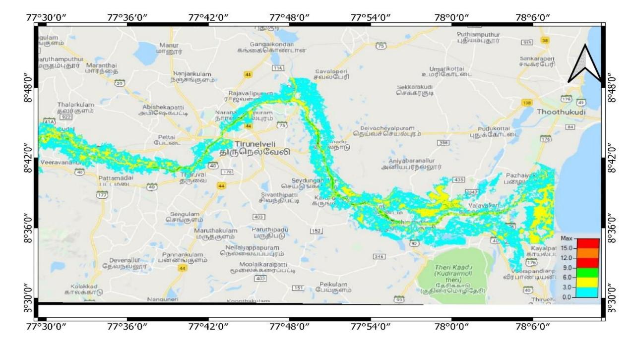
The flood inundation extent and the flood vulnerable areas can be found and merging the floodplain inundation model in a satellite imagery. The Highly vulnerable areas prone to flood are identified and located in the inundation map.
