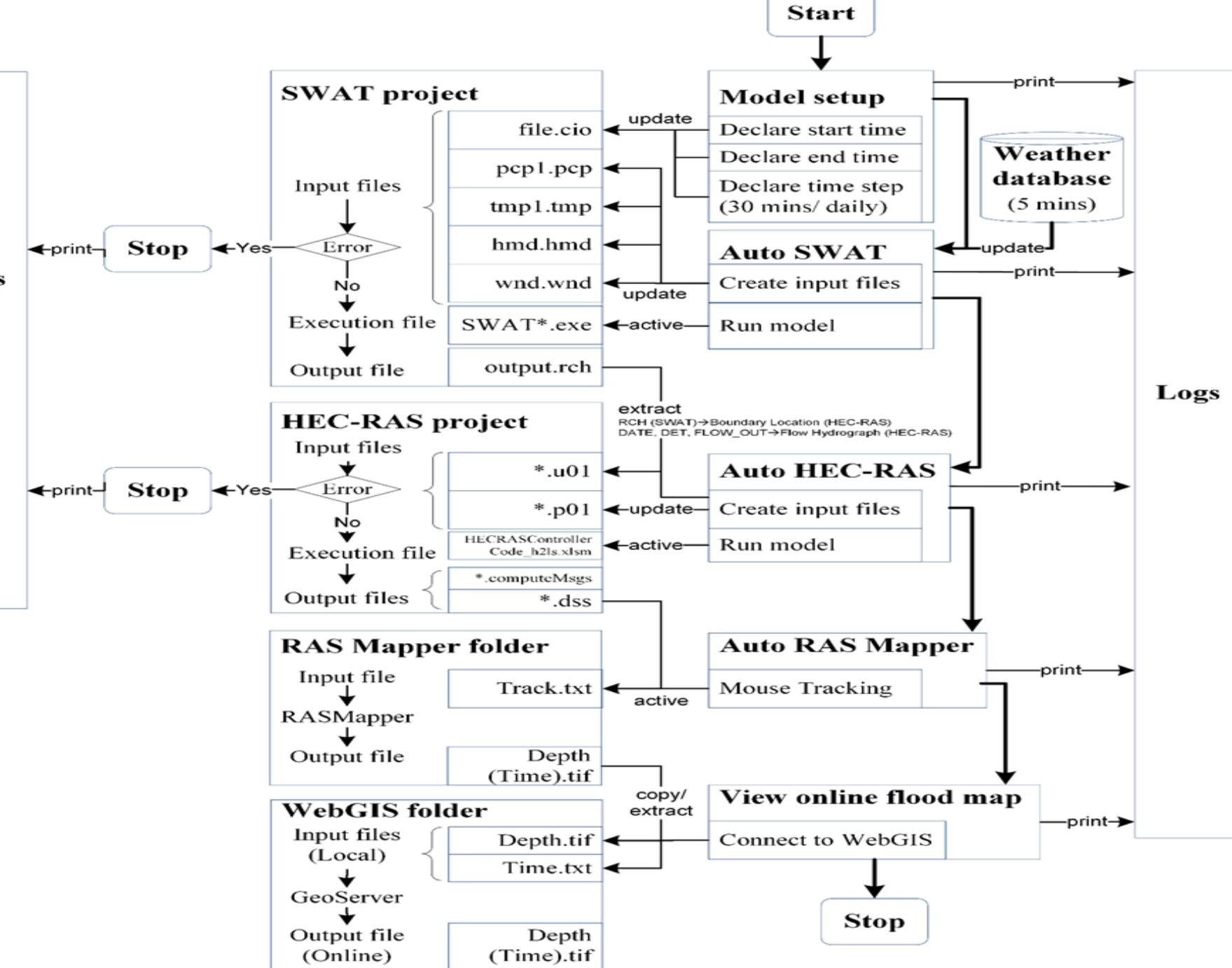
The flowchart of automated SWAT, HEC-RAS program for real-time flood forecasting
