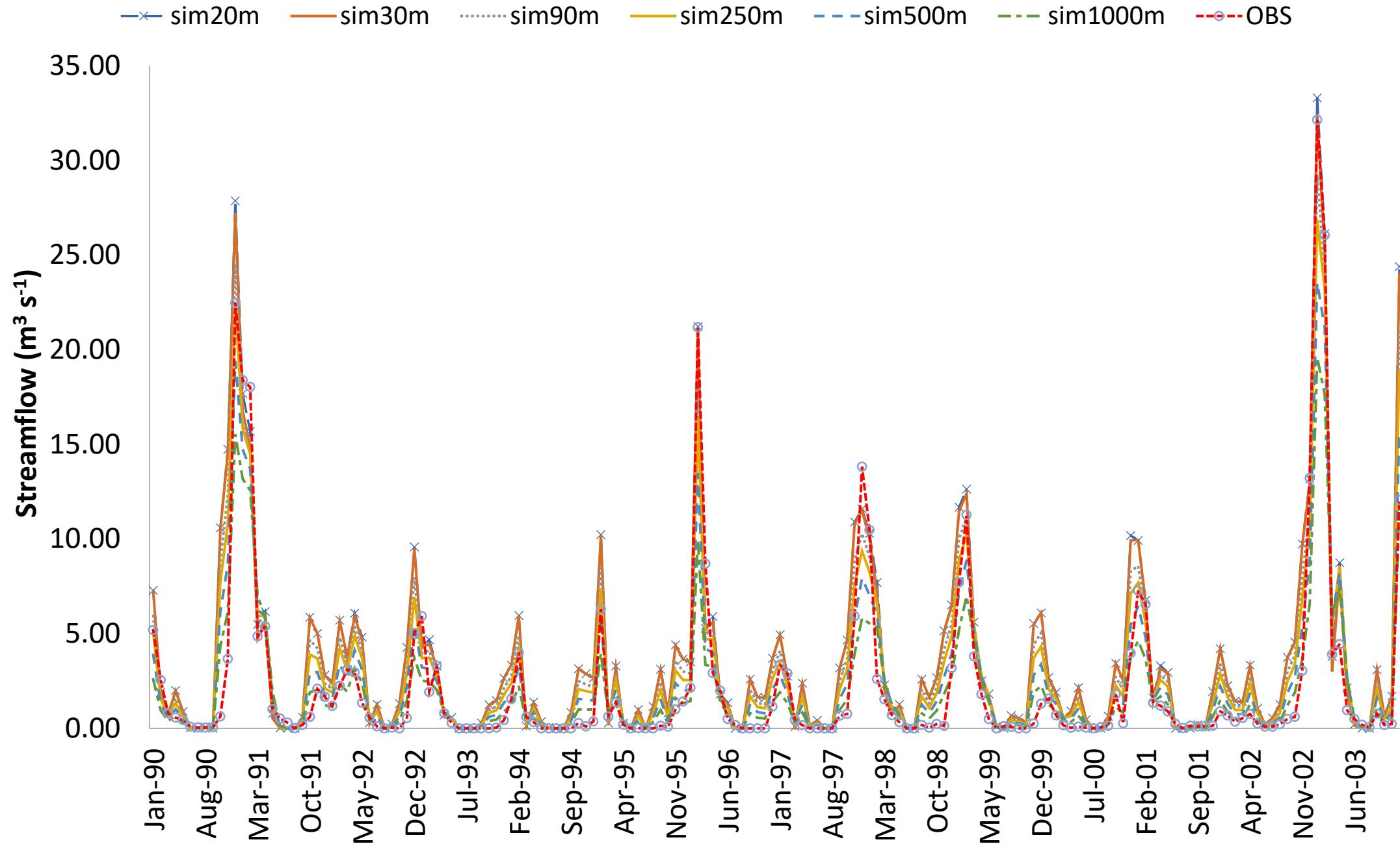
Results of performance criteria show that the use of finer resolution spatial data does not necessarily improve the performance of hydrological model predictions
