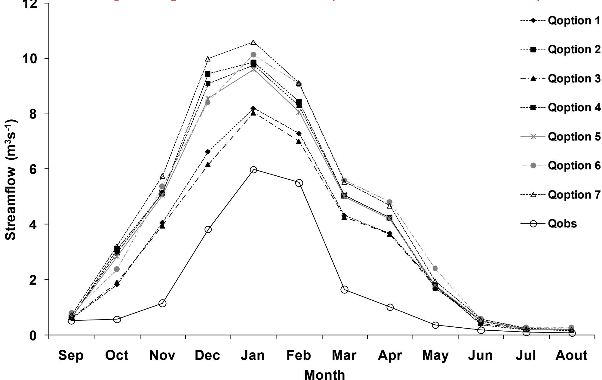
Predicted average monthly stream flow for each option and measured stream flow
