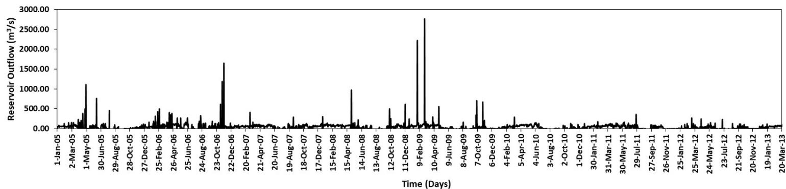
Figure 7. Daily reservoir outflow data at upper Indravati reservoir
