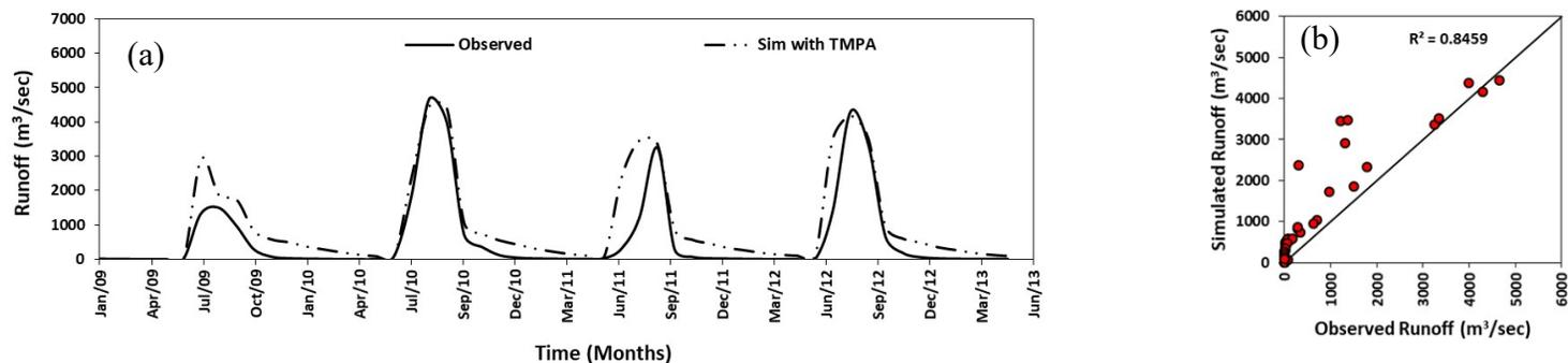
Figure 11. Monthly runoff estimated during validation period using SWAT model with considering reservoir
