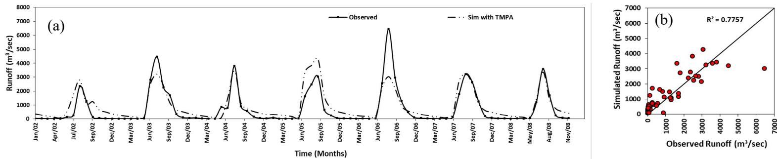
Figure 10. Monthly runoff estimated during calibration period using SWAT model with considering reservoir
