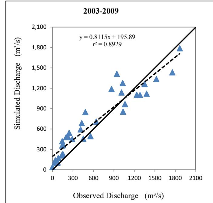
Simulation of monthly discharge  $\text{m}^3/\text{s}$
