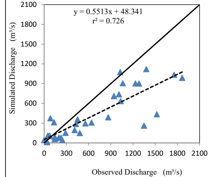
Statistical analysis of observed and Pre-calibrated simulated monthly discharge ( $\text{m}^3/\text{s}$ )
