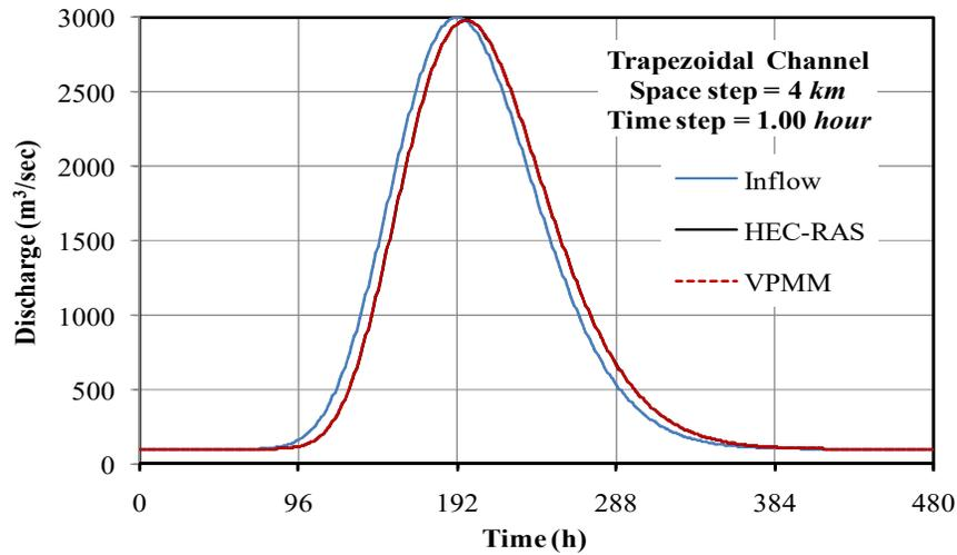
**Figure 5.** Typical simulated discharge hydrograph of the VPMM method for a space step of 4km and a time step of 1.00hour in a trapezoidal channel.
