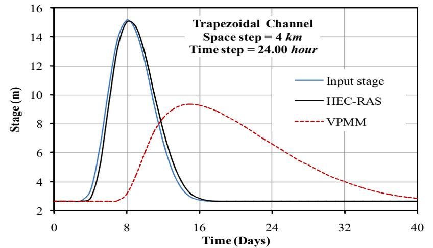
**Figure 8.** Typical computed stage hydrographs of the VPMM method for a space step of 4km and a time step of 24.00hour in a trapezoidal channel.
