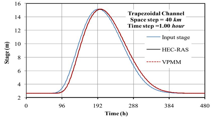
**Figure 2.** Typical computed stage hydrographs of the VPMM method for a space step of 40km and a time step of 1.00hour in a trapezoidal channel.
