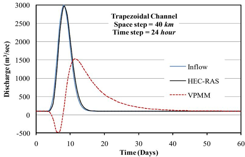
**Figure 3.** Typical simulated discharge hydrograph of the VPMM method for a space step of 40km and a time step of 24.00hour in a trapezoidal channel.
