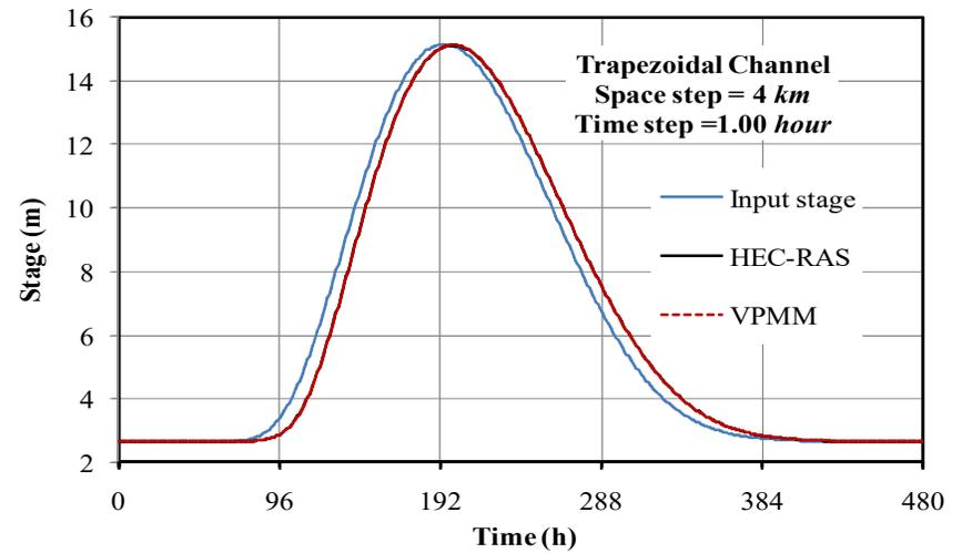
**Figure 6.** Typical computed stage hydrographs of the VPMM method for a space step of 4km and a time step of 1.00hour in a trapezoidal channel.
