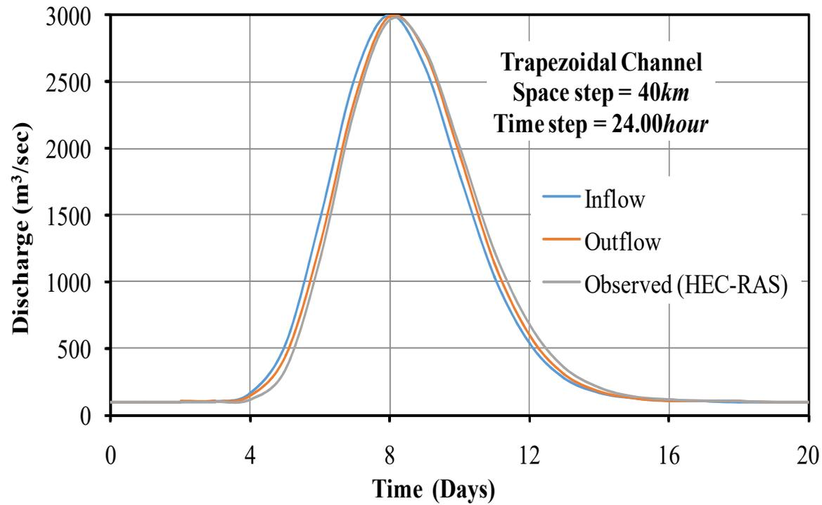
**Figure 13.** Typical computed discharge hydrographs of the constant-parameter method for a space step of  $40\text{km}$  and a time step of  $24.00\text{hour}$  in a trapezoidal channel using reference discharge
