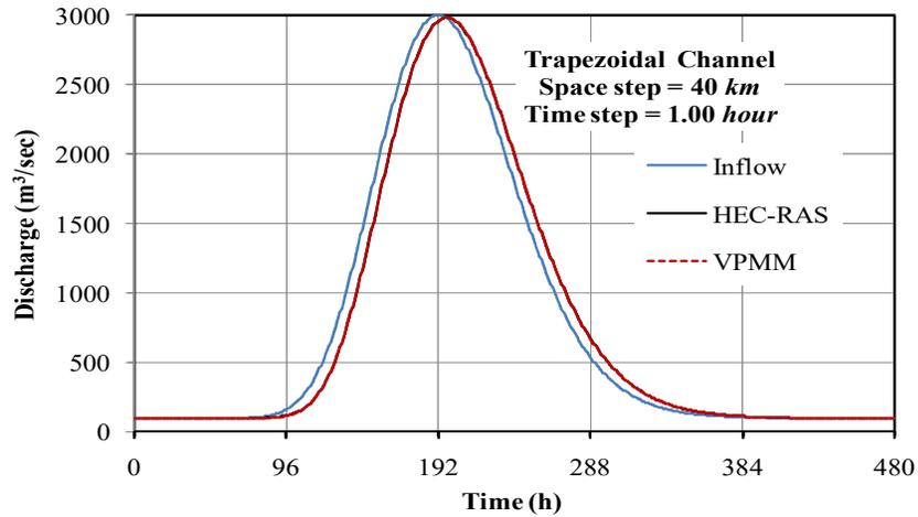
**Figure 1.** Typical simulated discharge hydrograph of the VPMM method for a space step of 40km and a time step of 1.00hour in a trapezoidal channel.
