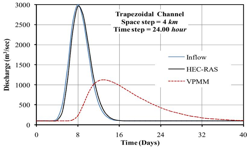
**Figure 7.** Typical simulated discharge hydrograph of the VPMM method for a space step of 4km and a time step of 24.00hour in a trapezoidal channel.
