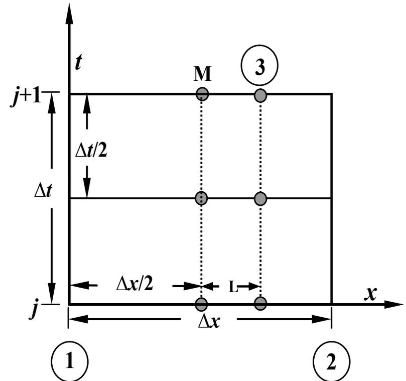
Fig. 2 Numerical grid adopted for VPMM application in synchronization with Fig.1
