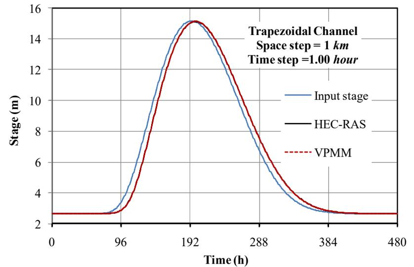
**Figure 10.** Typical computed stage hydrographs of the VPMM method for a space step of 1 km and a time step of 1.00 hour in a trapezoidal channel.
