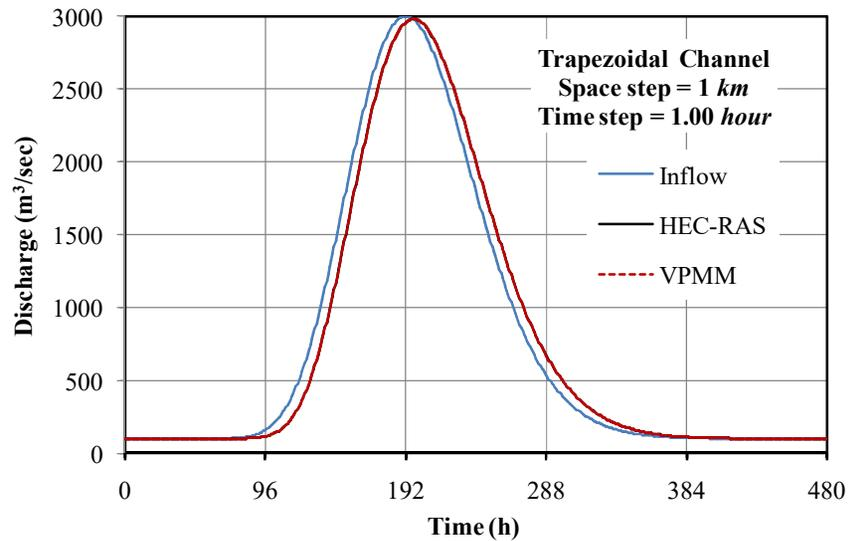
**Figure 9.** Typical simulated discharge hydrograph of the VPMM method for a space step of 1 km and a time step of 1.00 hour in a trapezoidal channel.
