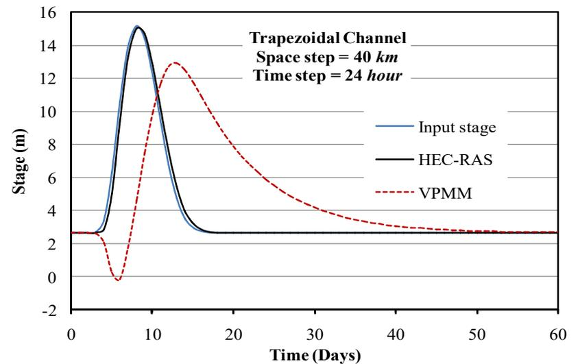
**Figure 4.** Typical computed stage hydrographs of the VPMM method for a space step of 40km and a time step of 24.00hour in a trapezoidal channel.
