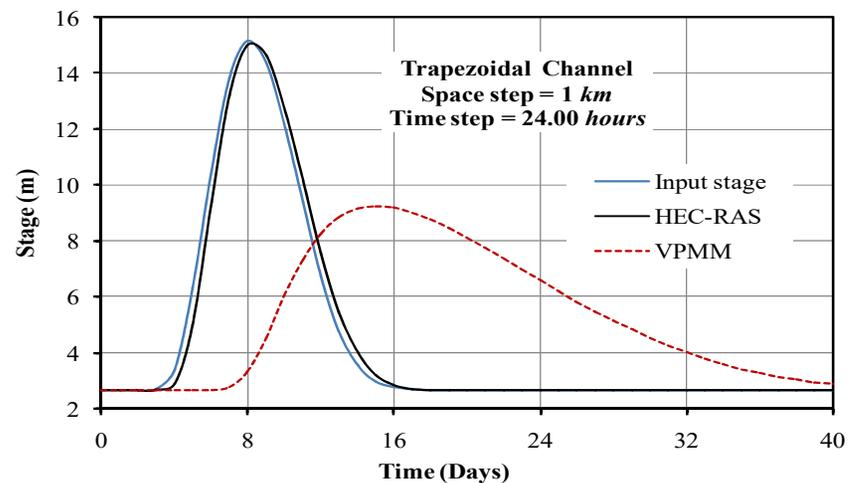
**Figure 12.** Typical computed stage hydrographs of the VPMM method for a space step of 1 km and a time step of 24.00 hour in a trapezoidal channel.
