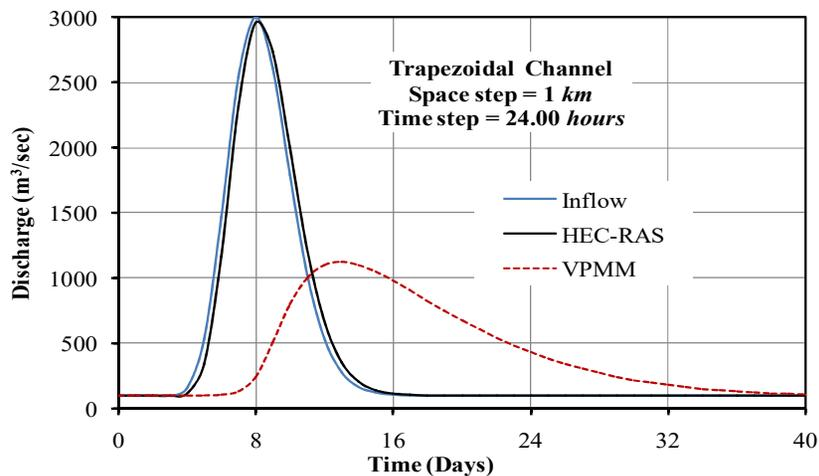
**Figure 11.** Typical simulated discharge hydrograph of the VPMM method for a space step of 1 km and a time step of 24.00 hour in a trapezoidal channel.
