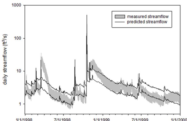
**Figure 1 – Measured and simulated daily streamflow hydrograph for the Medina River (from Harmel et al., 2010). The uncertainty boundaries are presented as the shaded area for measured streamflow and as the upper and lower boundary lines for simulated streamflow.**
