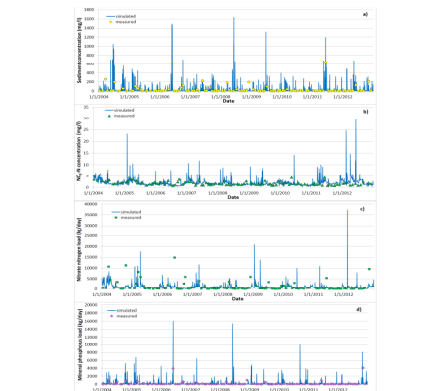
Figure 4: A comparison of the simulated and the calculated sediment load (a), nitrate-nitrogen concentration (b) and load (c) and phosphorus load (d) in the river Sotla for station Zelenjak at subbasin 6 outlet between 2004 and 2012
