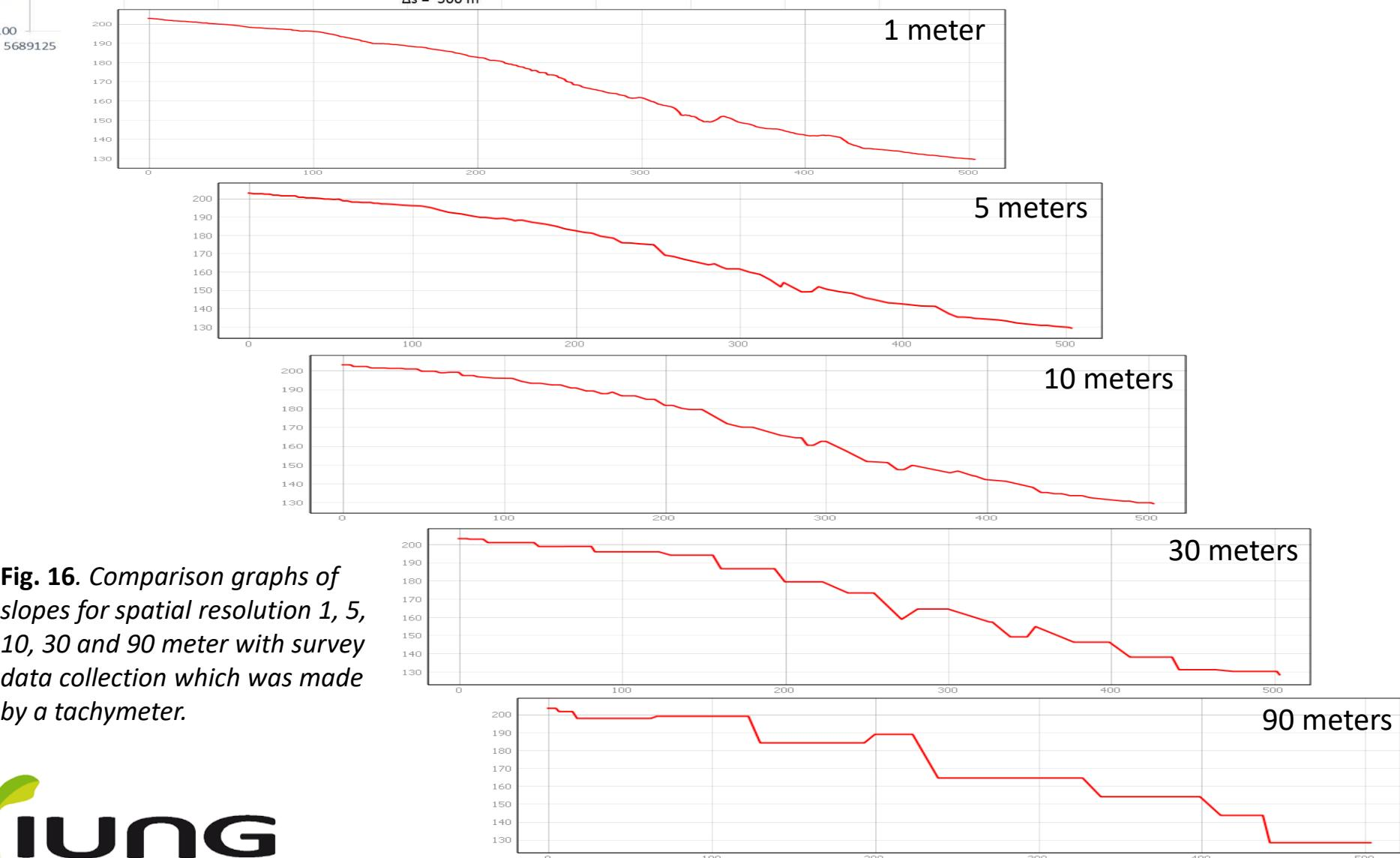
**Fig. 16.** Comparison graphs of slopes for spatial resolution 1, 5, 10, 30 and 90 meter with survey data collection which was made by a tachymeter.
