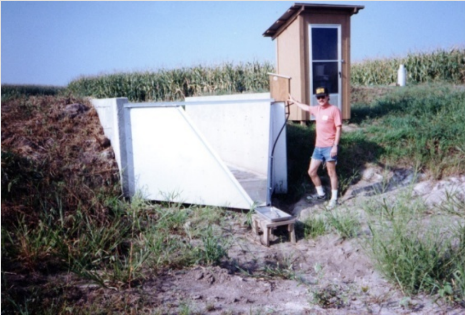
Each watershed is drained by a grass waterway, leading to a concrete approach structure and H-flume
