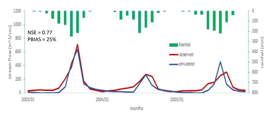
SWAT model calibration was done using streamflow at the Pwalugu river gauging station in White Volta.
