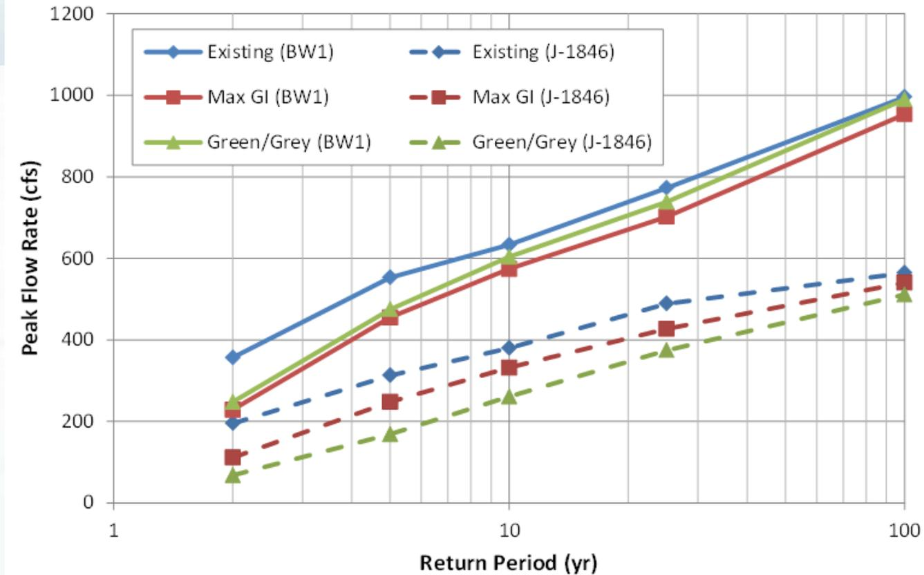
**1D Design Storm Peak Flow Rates at Watershed Outlet (BW1) and Interior Node (J-1846 in Channel North of Arcadia Ave)**
