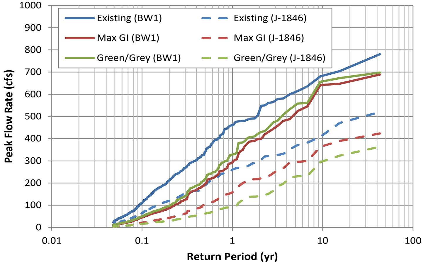
**1D Continuous Simulation Peak Flow Rates at Watershed Outlet (BW1) and Interior Node (J-1846 in Channel North of Arcadia Ave)**
