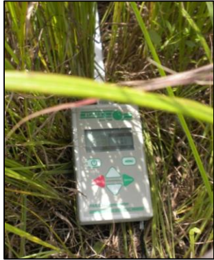
Decagon Devices, AccuPAR LP-80, Adapted Plant /Transect Method (Johnson, Kiniry, Burson, 2010)
