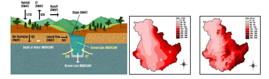
A module for simulating paddy rice fields was added to SWAT, and linked to MODFLOW for simulating surface-ground water interaction with fully-coupled manner. GW module of SWAT was replace by MODFLOW.
