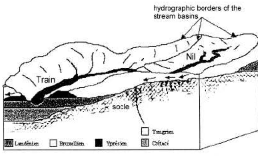
The Nil basin has groundwater loss through sand layers towards the catchment of the Train. The base flow is very low.
