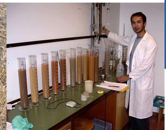
Physical Parameters: Ksat, Bulk Density and Particle Size Distribution.
