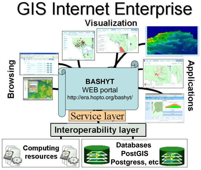
BASHYT has a layered structure (interoperability layer, service layer, application layer, etc.), and is built with open source technologies (no limitation of commercial products)
