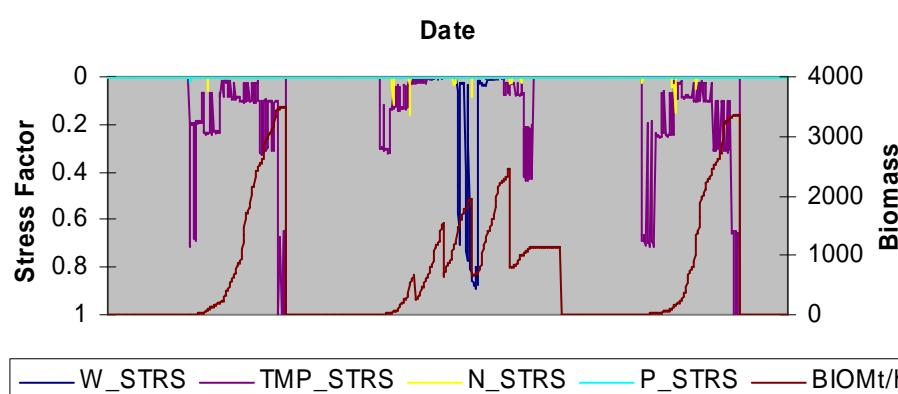
CSIL alternated with CVLR on HRU 38 in SUB 38: Biomass versus Stress Factors (1985-1986-1987)
