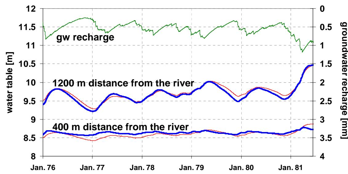
Comparison of groundwater table dynamics calculated by the simplified linear groundwater model (based on the Hooghoudt-Equation) and a numerical solution of the non-linear Boussinesq-Equation under well defined boundary conditions.
