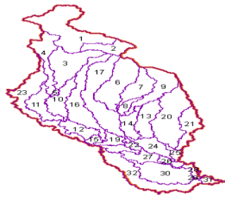
Figure 7. Delineated Bagmati basin and its sub-basins
